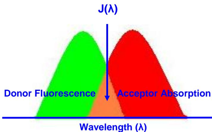
**Figure 2.** Schematic representation of the FRET spectral overlap integral
