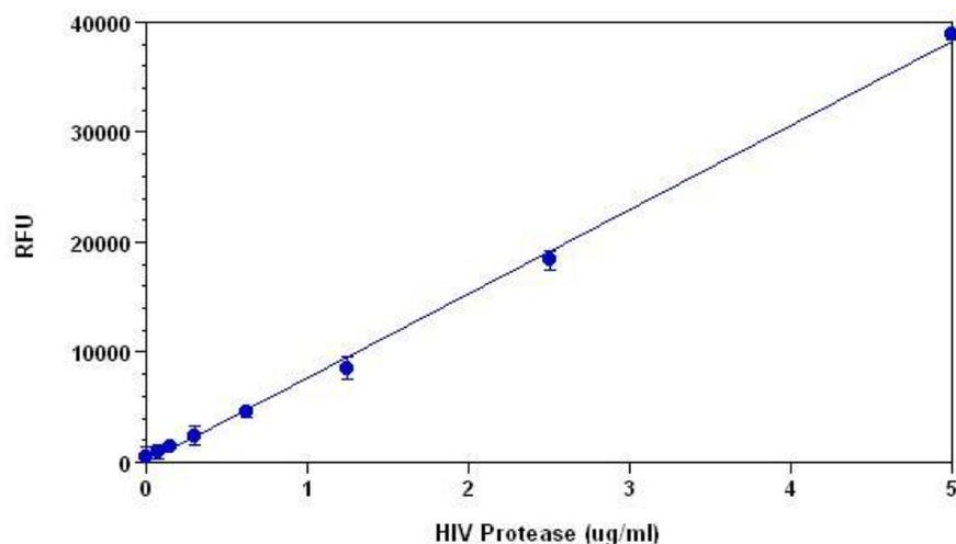
**Figure 5.** HIV Protease cleavage of Tide Fluor™ 2/Tide Quencher™ 2-derived FRET peptide. Upon cleavage, the fluorescence of Tide Fluor™ 2 is recovered, and can be monitored at EX/EM = 490/520 nm. With excellent fluorescence quantum yield and longer excitation and emission wavelength, the fluorescence signal of Tide Fluor™ 2 is less interfered by the autofluorescence of cell components and test compounds, thus providing better assay sensitivity.
